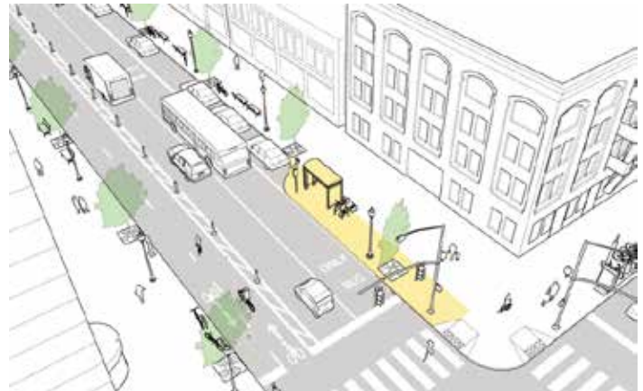
Figure 9: Example of a transit bump-out Source: NACTO Urban Street Design Guide
