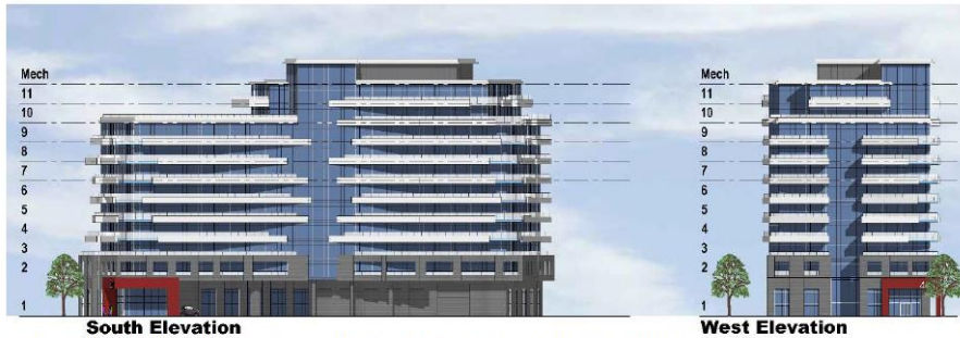
South and West Elevations showing stepped profile from 11 to 9 storeys and balcony articulation.
