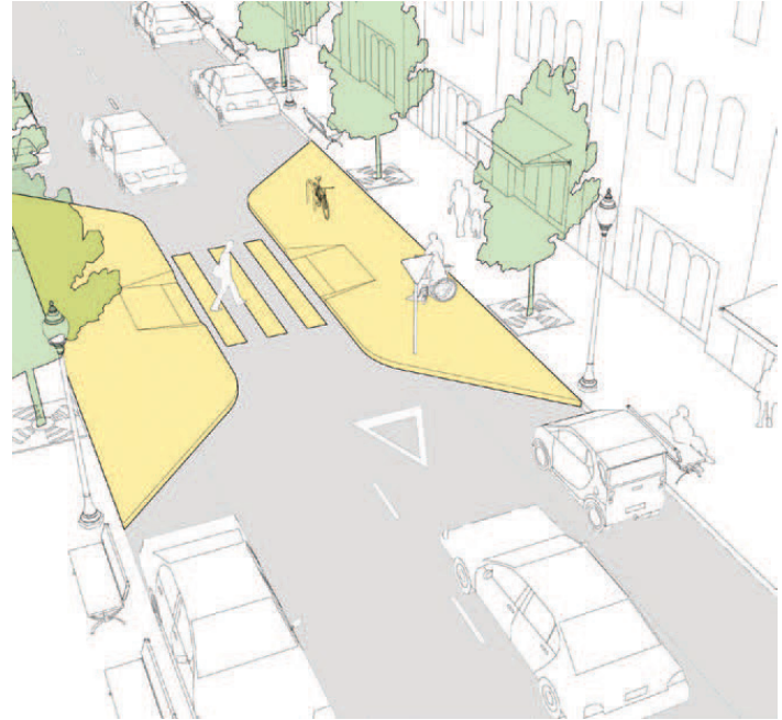
Figure 8: Example of a mid-block bump-out treatment Source: NACTO Global Street Design Guide
