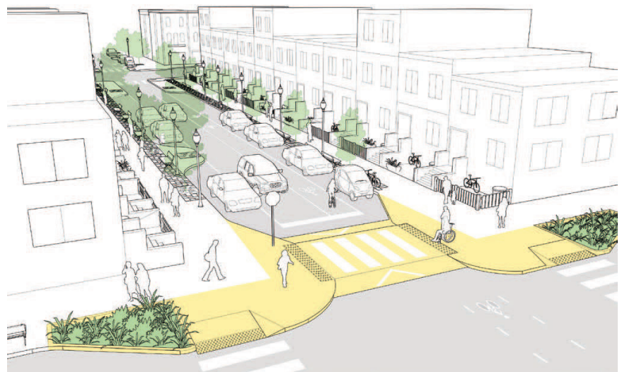
Figures 4 & 5: Examples of gateway and node intersection treatments Source: NACTO Global Street Design Guide
