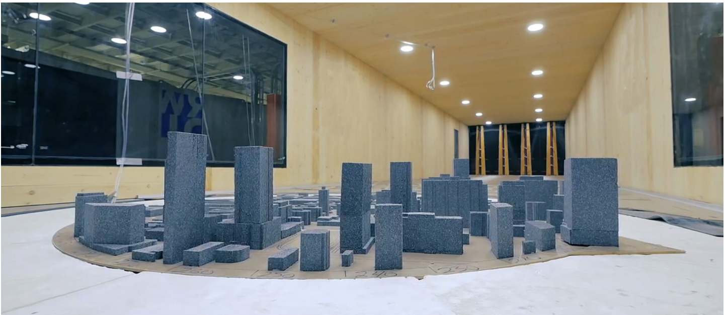
Figure 3.3 - Building model in a wind tunnel facility
