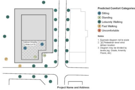
Example Wind Tunnel Test Sensor Location Plan and Predicted Pedestrian Wind Comfort Criteria
