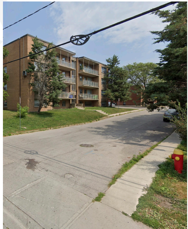
Private streets should provide at least one sidewalk between 1.5 to 2.0 metres in width
