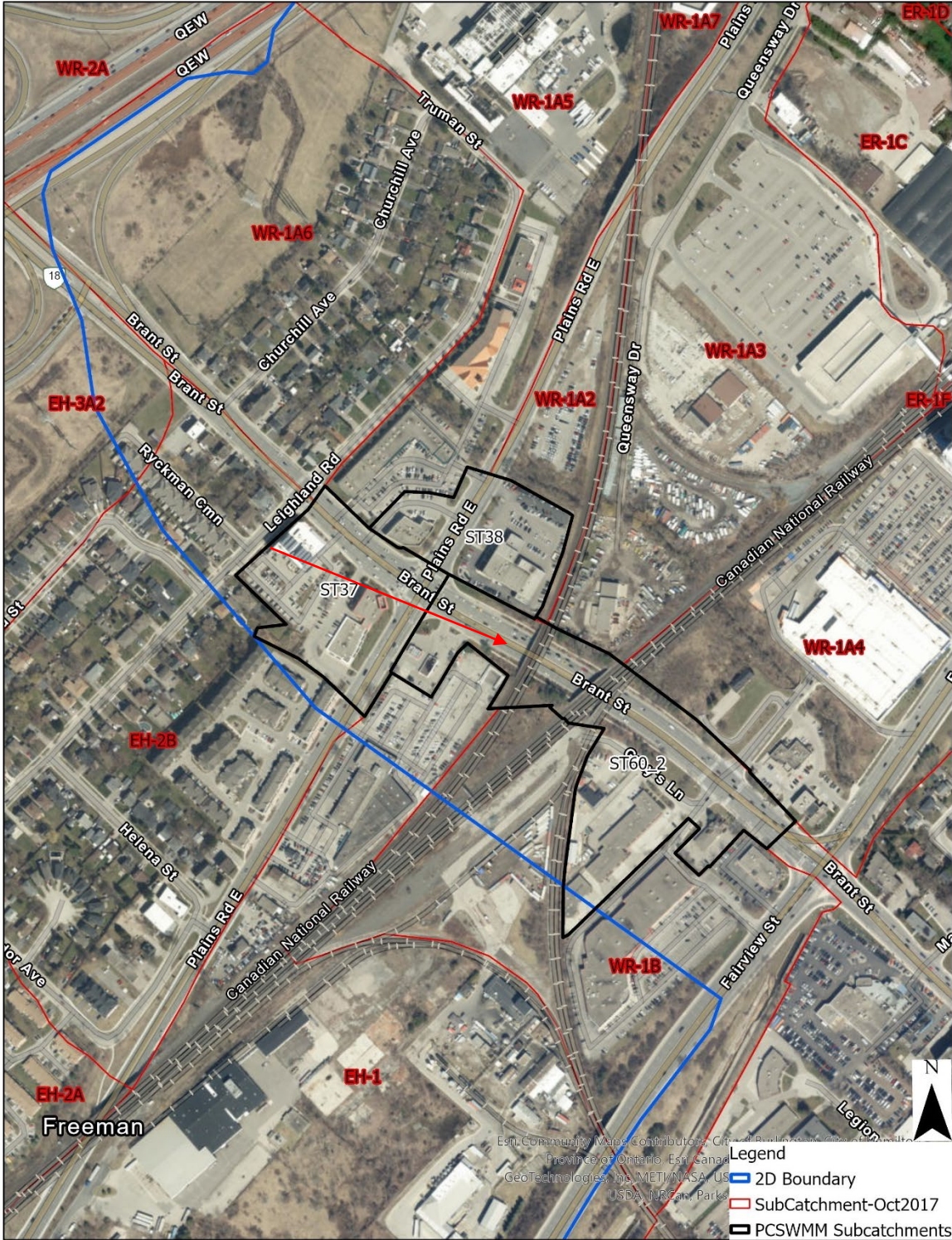
Figure 2.2.10. Inflow into the Brant Street Underpass Subcatchment (from PCSWMM)
