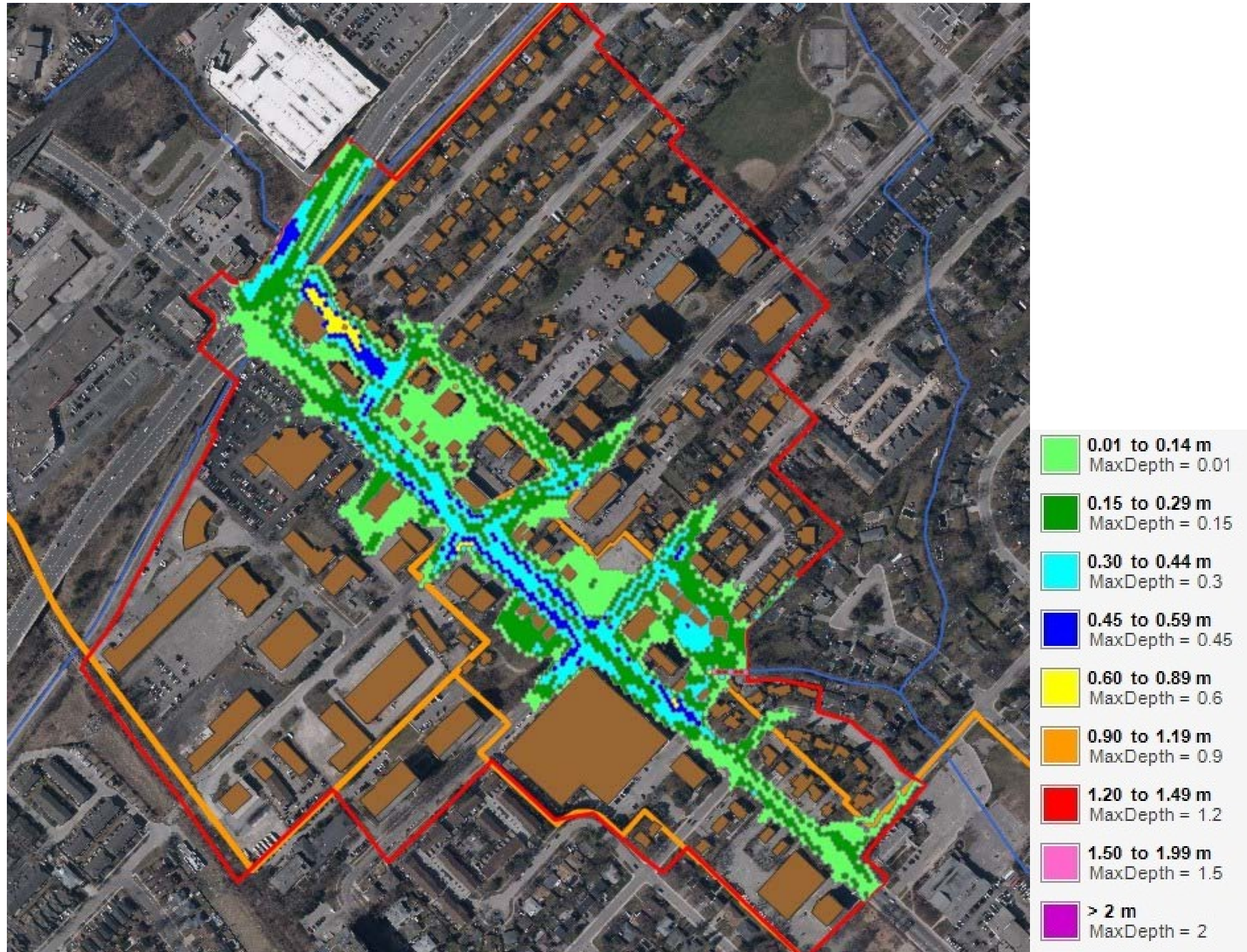
Figure 2.12: 2D Modelled Maximum Depth Contours for areas Downstream of Fairview Street (Spill Scenario 4 - Regional Storm Event, Scenario 1)
