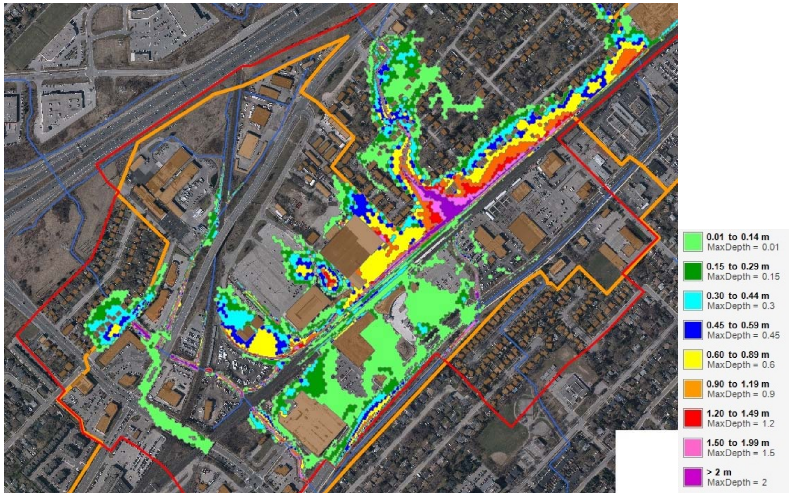
Figure 2.7: 2D Modelled Maximum Depth Contours for West Rambo and East Rambo Creek areas between the QEW and Fairview Street (Regional Storm Event, Scenario 2)
