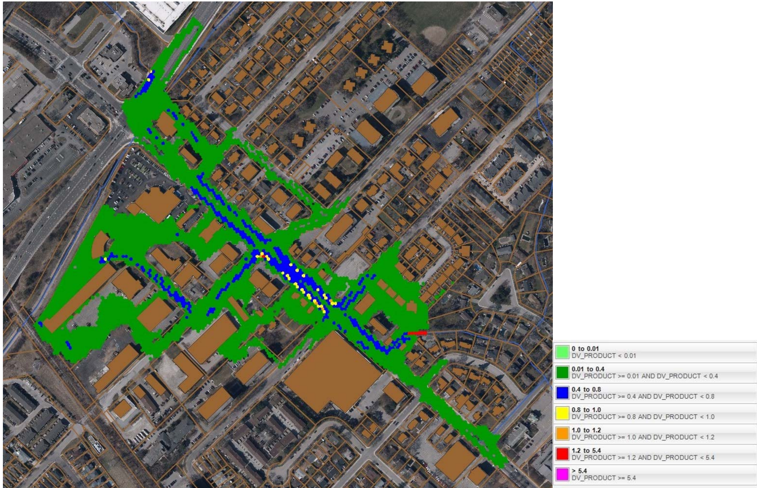
FIGURE C12: 2D MAXIMUM DEPTH X VELOCITY SUMMARY FOR HAGER-RAMBO DIVERSION CHANNEL SPILLS – REGIONAL STORM (SCENARIO 2)
