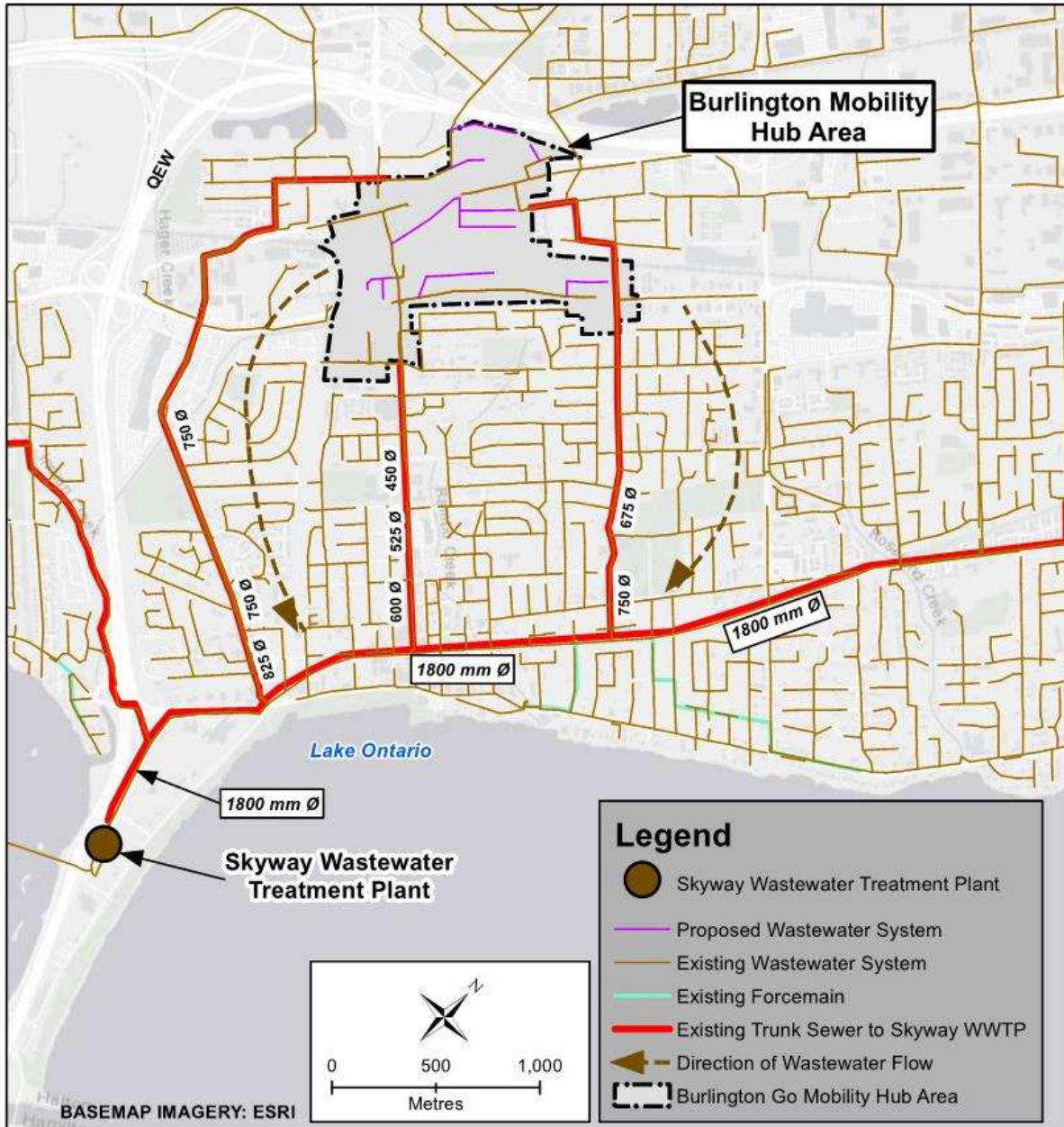
Figure 3-3. Existing Wastewater Services Burlington Go MTSA
