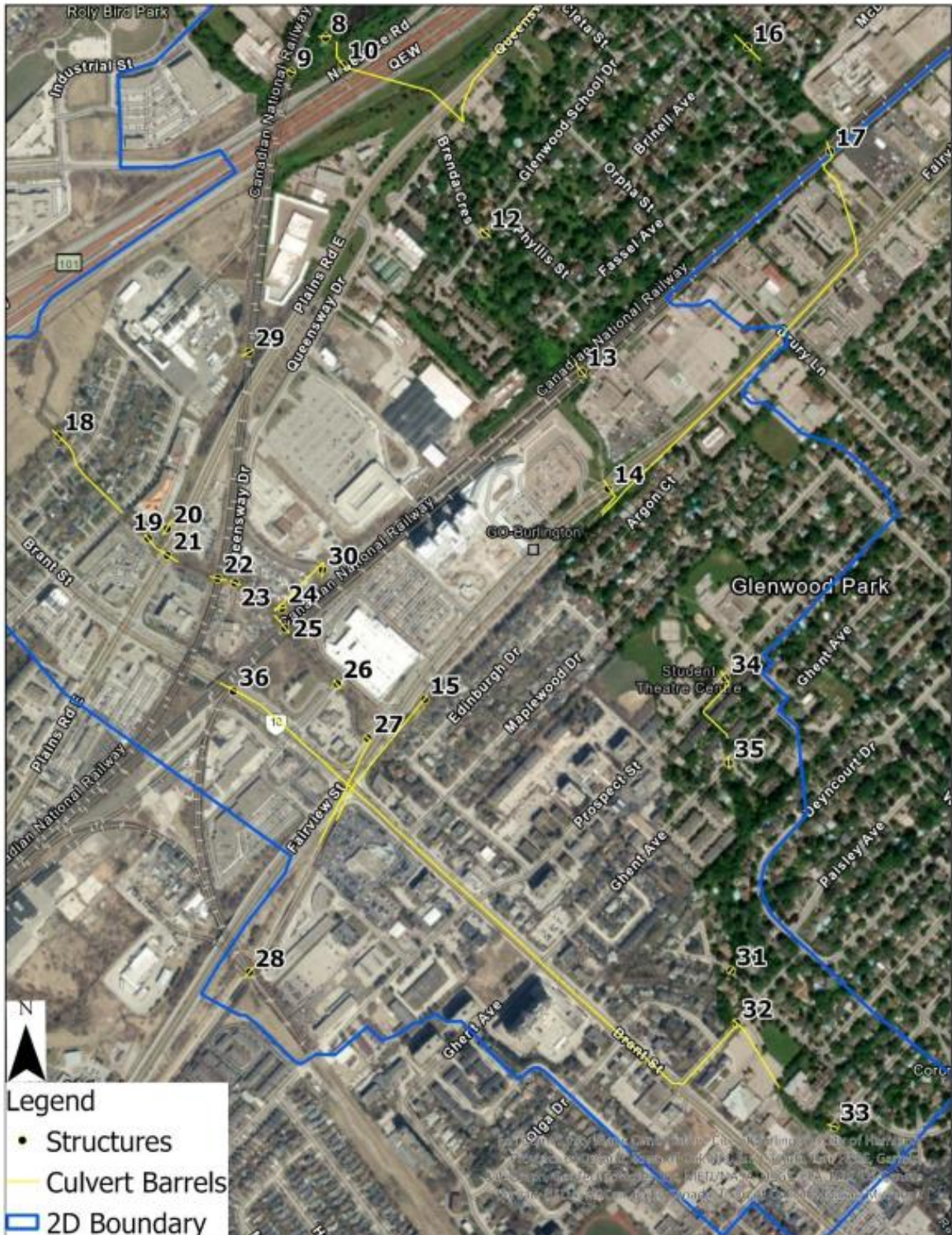
Figure R1: Culvert Locations (Rambo Creek)
