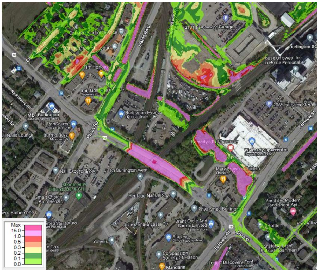
Figure R2: Simulated Regional Storm Floodplain and Spill with Rambo Creek Culvert Improvements in Place
