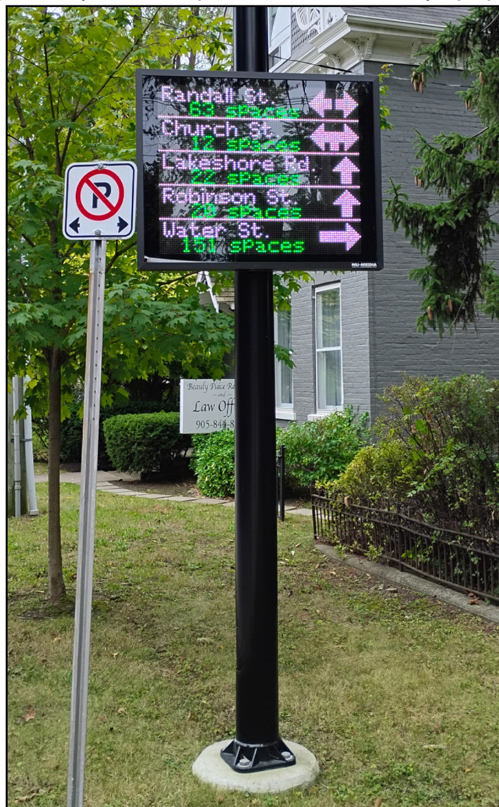
Figure 38: Dynamic Parking Lot Location and Availability Signage
